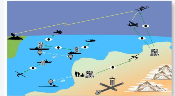
Operational View (OV-1) shows line-of-sight (LOS) optical signaling via Quick Reaction (QR) codes and Digital Flashing Light (DFL). Only two radio frequency (RF) lightning bolts!
