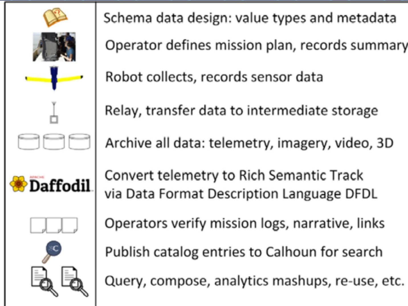
*Robodata Workflow: collection and storage of data enables recording, replay, smoothing and visualization of robot tracks.*
